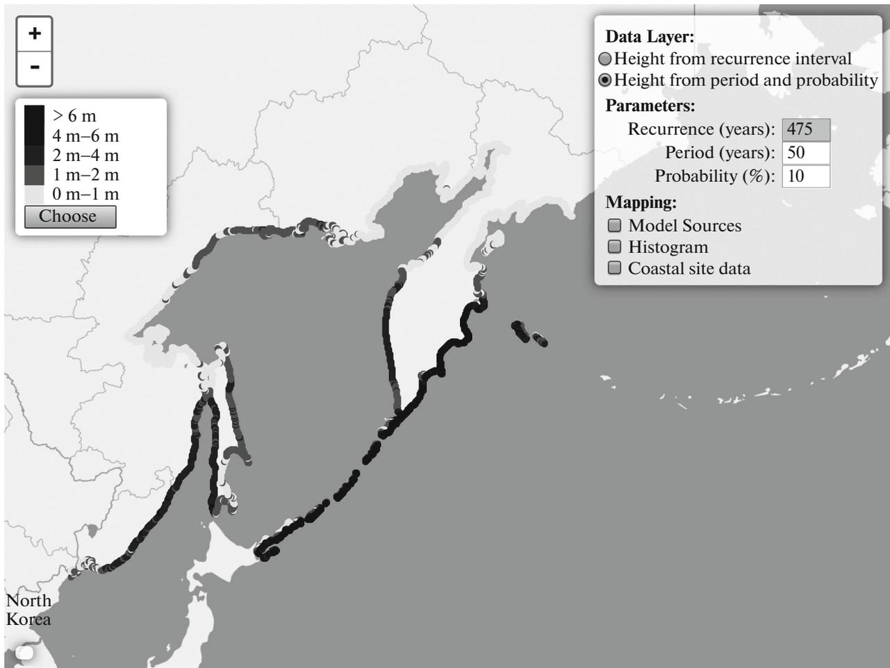
**Fig. 3.** An example of the calculated tsunami hazard map for the Far Eastern coast of the Russian Federation obtained in the framework of the PTHA methodology:  $P = 10\%$ ,  $T = 50$  years, recurrence interval of one time in 475 years.
