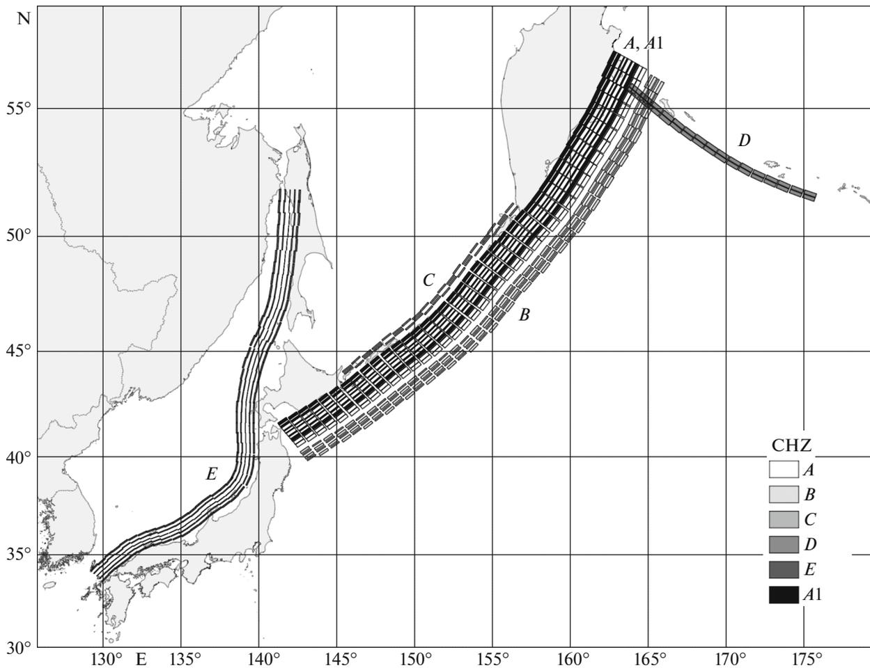
**Fig. 1.** The fault plane projections in the sources of model earthquakes with magnitude  $M_w = 7.2$  in conditionally homogeneous zones.
