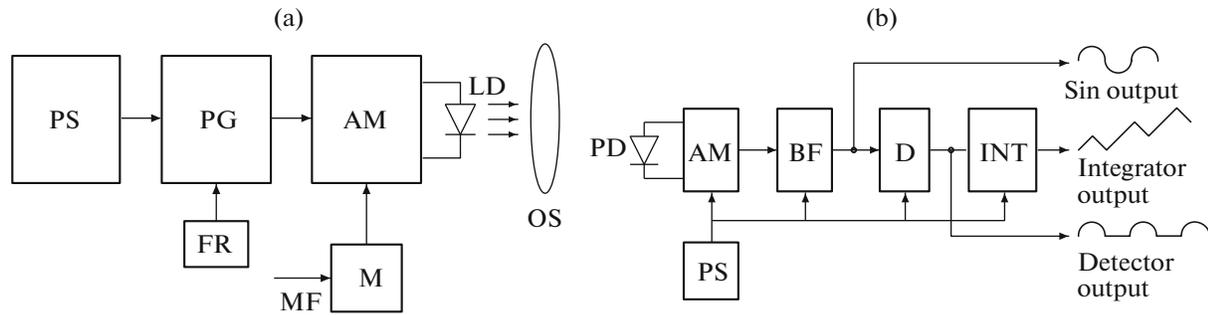
**Fig. 2.** Scheme of the optical bench: block diagrams of the (a) optical pulse radiator module and (b) optical receiver. Notation: PS is the power source, AM is the amplifier, M is the modulator, MF is the modulating frequency, LD is the laser semiconductor diode, OS is the optical system, PD is a photodiode, BF is the bandpass filter, and D is the detector.
