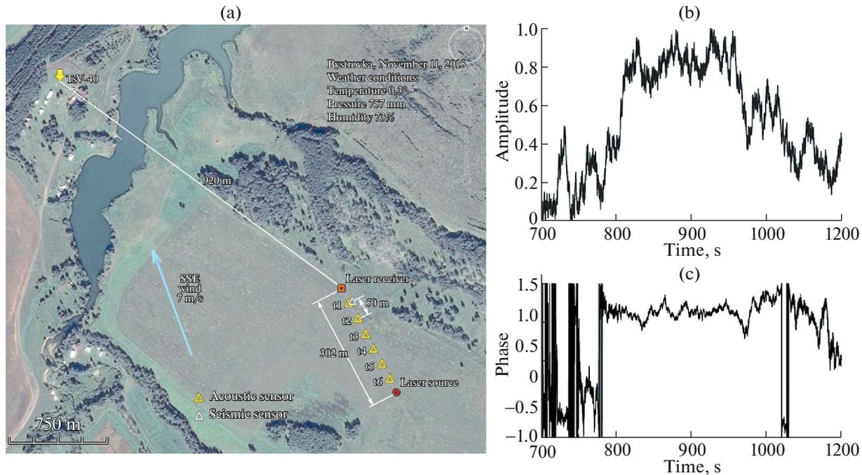
**Fig. 5.** Scheme of the field experiment and its results: (a) map of the terrain and arrangement of units of the acoustooptical system and TsV-40 vibrator in the region of the Bystrovka test area; (b) result of processing of optical oscillations in the measuring beam: amplitude accumulation of the envelope due to the presence of an external acoustic oscillation with a frequency of 9.5 Hz; and (c) is the established oscillation phase complicated by noises.
