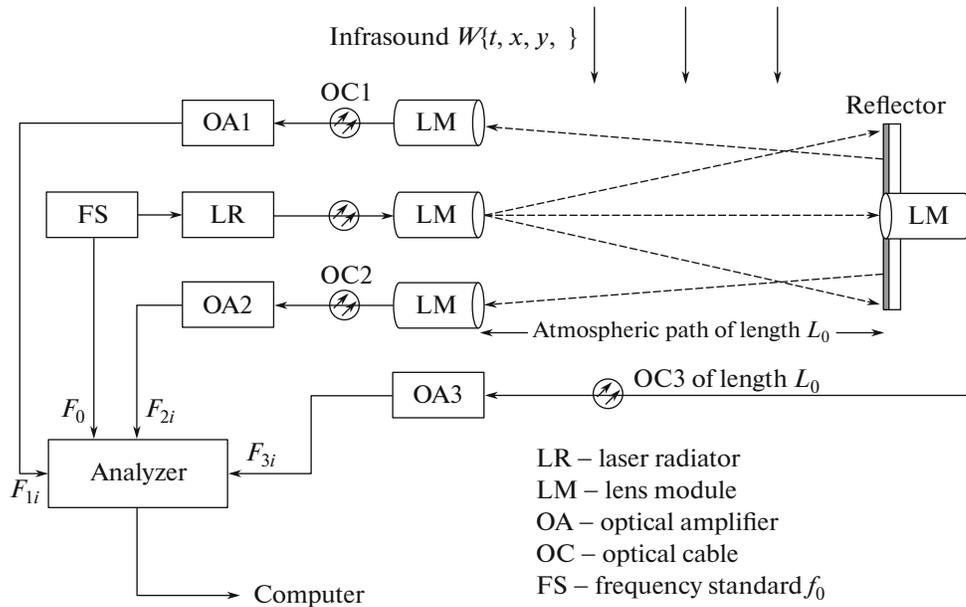
Fig. 6. Structure of the scheme of measurements with the frequency method for infrasound monitoring.
