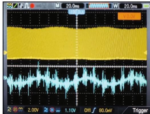
**Fig. 3.** Waveform of an AM signal of radiation with a modulation depth of 5.1% (in the upper part of the figure) and its envelope from the output of the optical receiver (in the lower part of the figure) on a 80-m-long path.
