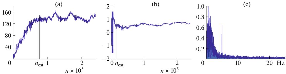
**Fig. 4.** Results of digital processing of an optical signal: (a) current value of the amplitude, (b) phase, and (c) spectrum of the optical signal envelope at a modulation depth of 0.4%.
