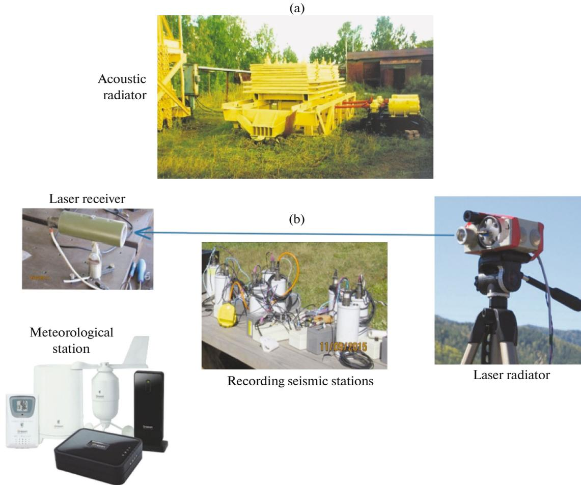
**Fig. 1.** Components of the acoustooptical system: (a) TsV-40 seismic vibrator and (b) optical bench.
