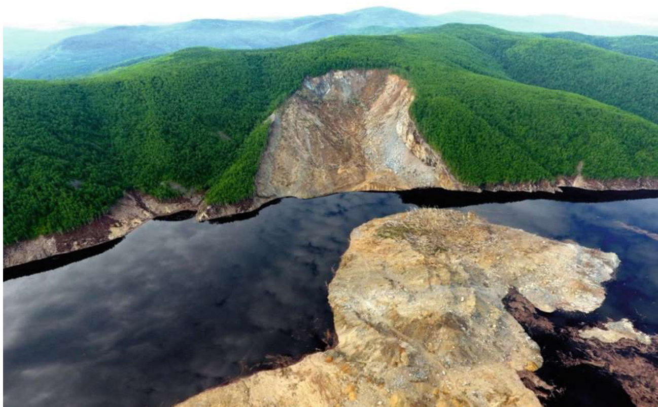
Fig. 3 General view of the landslide scar on the southern bank of the Bureya water reservoir and the body of the landslide with a passage, initially made in February 2019 and then extended by the spring flood
